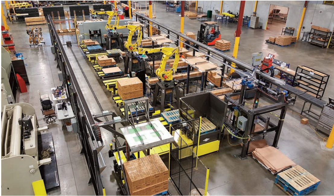
Nine line palletizers show full automation with robots having a starring role in the process.
