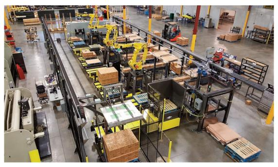
Nine line palletizers show full automation with robots having a starring role in the process.
