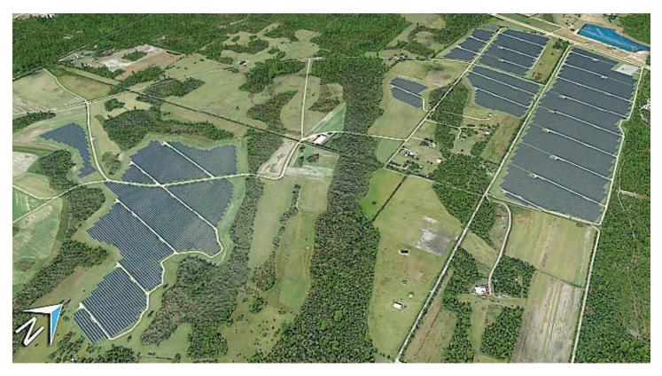
FPL Pioneer Trail Solar Energy Center in Samsula includes 350,000 photovoltaic solar panels installed on 436 acres.
